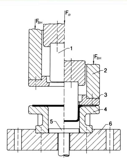
If D/s < 20 (thick sheet), no blank holder is needed.
