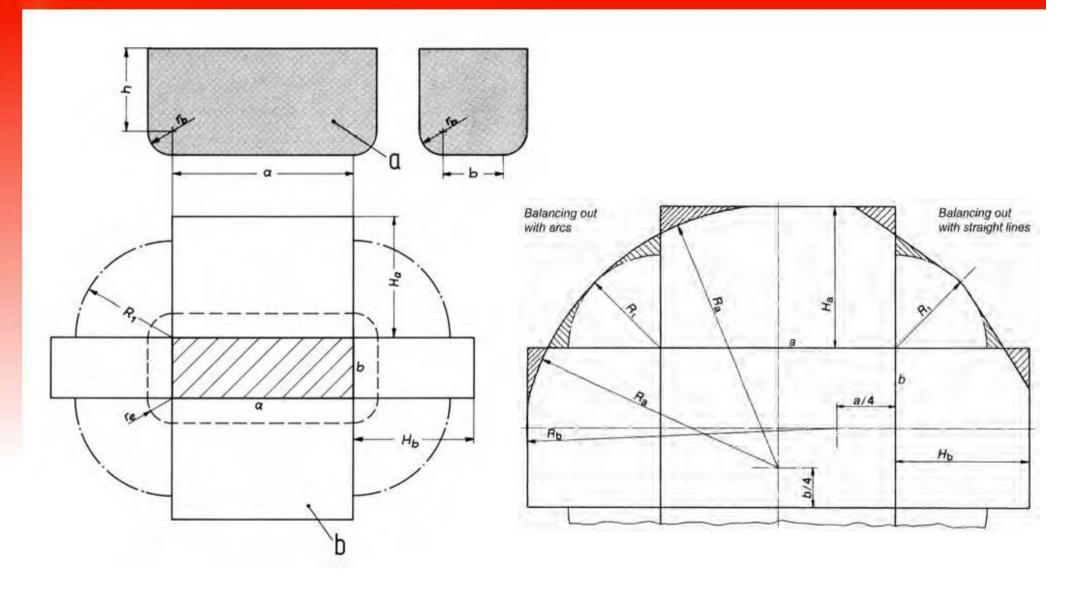
Breakdown of a rectangular hollow part into elements of equal area
